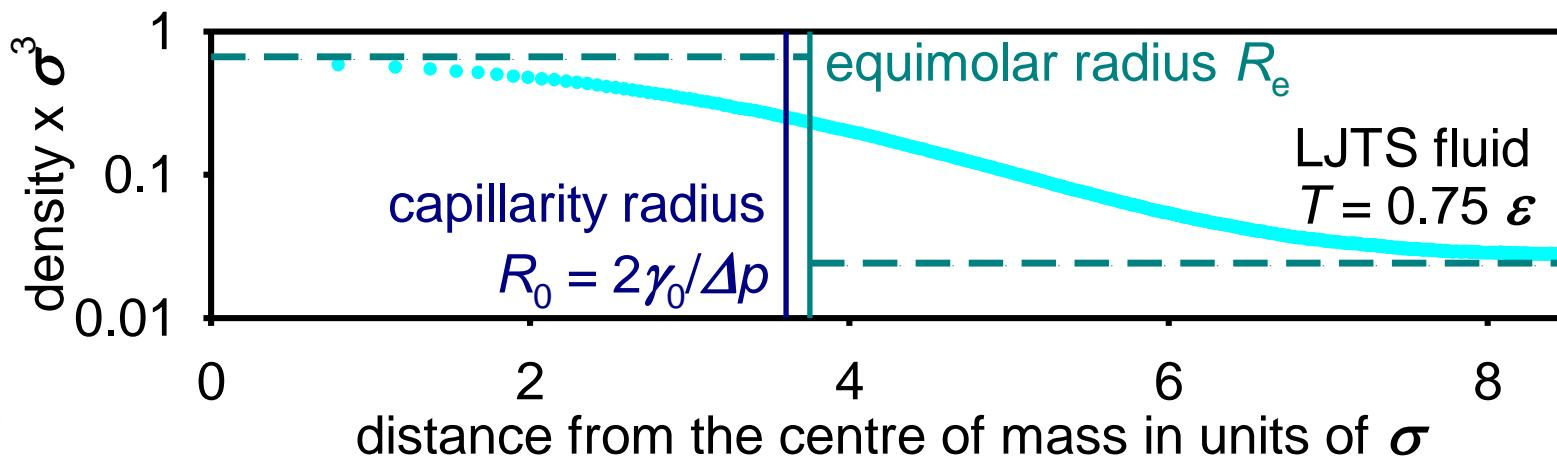
Novel approach: Use  $\Delta p$  instead of  $1/R_L$ , use  $R_0 = 2\gamma_0/\Delta p$  instead of  $R_L$ .
