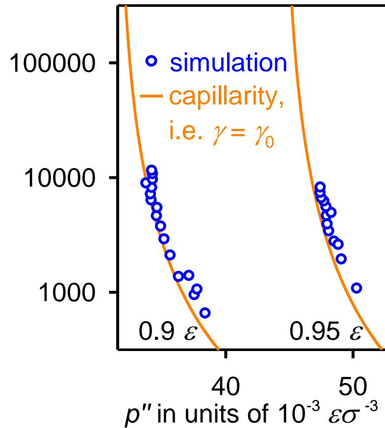
Simulation results support the capillarity approximation for  $n > 1\,000$ .
