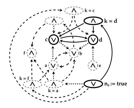
By disabling as many nodes as possible, the **deletion algorithm** finds  $T_s = \{c, d\}$ , the minimal statically stubborn set at  $\mathfrak{m}_0$ .
