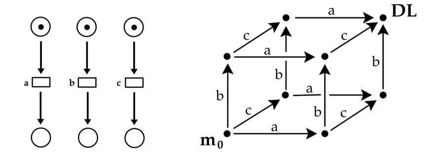
A net composed of  $\mathfrak n$  parallel nets, each with k reachable components, has a total of  $k^n$  states.
