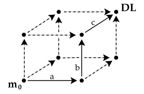
The remaining subset of T is called **stubborn** at  $\mathfrak{m}_c$ . In general, for every marking  $\mathfrak{m}_c$  reached while exploring the state space, we try to eliminate as many transitions as possible.
